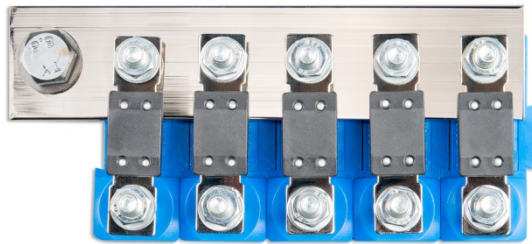
Stacked fuse holders with 5-position high current bus bar (copper 40 x 5 mm)
