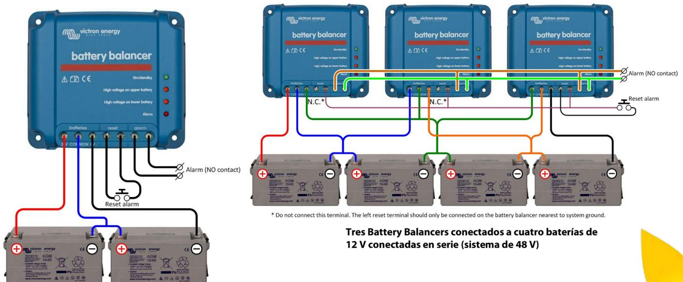
\* Do not connect this terminal. The left reset terminal should only be connected on the battery balancer nearest to system ground.
